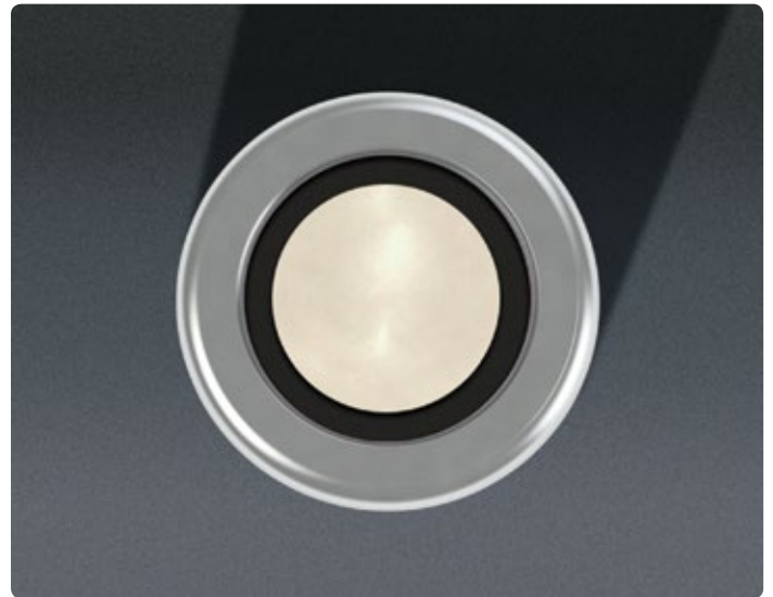
Figure 10. Used Cap exposed to strong oxidizers is bleached white and emits no color.
