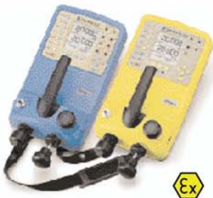
Portable Pressure Calibrators DPI 615/DPI 615IS
